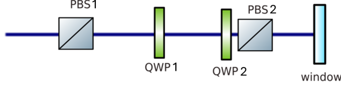
Figure 5.1. Simplified schematics of the setup used to tune the circular polarization.
