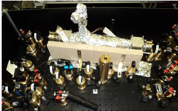
Figure 3.6: Picture of the SAS cell on its own optical table. The cell is wrapped with a heating tape and then insulated with fiberglass tape and aluminum foils. Thermal bricks have been put close to it to reduce heating of the optical system.
