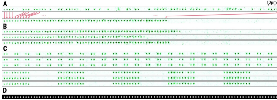
Figure 2.3: Rearrangement of arrays of optical tweezers in arbitrary patterns. Defect free 1D array rearranged using one AOD. Image taken from [28].
